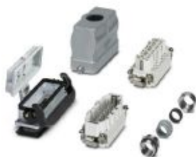
Connector set, consisting of: B16 sleeve housing and panel mounting base, 16-pos. plug and socket insert, M25 cable gland
