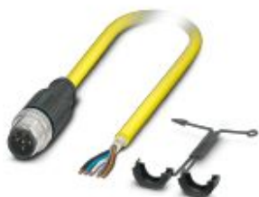
Sensor/actuator cable, 5-position, PVC, yellow, shielded, Plug straight M12, coding: A, on free cable end, cable length: 5 m
