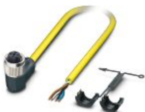
Sensor/actuator cable, 4-position, PVC, yellow, free cable end, on Socket angled M12 SPEEDCON, coding: A, cable length: 2 m
