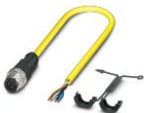
Sensor/actuator cable, 4-position, PVC, yellow, Plug straight M12 SPEEDCON, coding: A, on free cable end, cable length: 5 m
