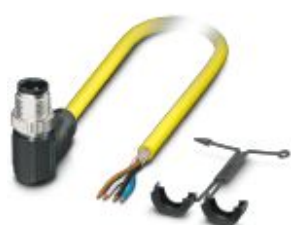
Sensor/actuator cable, 4-position, PVC, yellow, shielded, Plug angled M12, coding: A, on free cable end, cable length: 5 m
