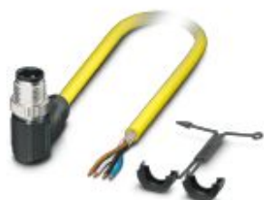
Sensor/actuator cable, 4-position, PVC, yellow, shielded, Plug angled M12, coding: A, on free cable end, cable length: 10 m
