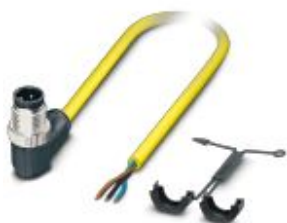
Sensor/actuator cable, 3-position, PVC, yellow, Plug angled M12 SPEEDCON, coding: A, on free cable end, cable length: 2 m
