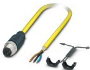
Sensor/actuator cable, 3-position, PVC, yellow, shielded, Plug straight M12, coding: A, on free cable end, cable length: 2 m
