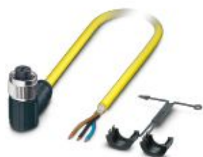
Sensor/actuator cable, 3-position, PVC, yellow, shielded, free cable end, on Socket angled M12, coding: A, cable length: 5 m
