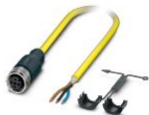
Sensor/actuator cable, 3-position, PVC, yellow, shielded, free cable end, on Socket straight M12, coding: A, cable length: 10 m
