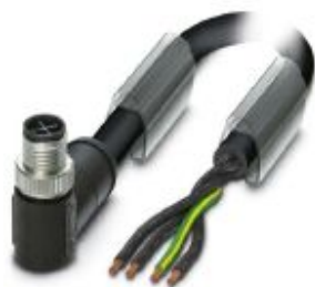
Power cable, 4-position, PUR halogen-free, black-gray RAL 7021, Plug angled M12, coding: S, on free cable end, cable length: 10 m, for AC current up to 12 A/690 V
