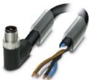
Power cable, 4-position, PUR halogen-free, black-gray RAL 7021, Plug angled M12, coding: T, on free cable end, cable length: 2 m, For direct current up to 12 A/63 V
