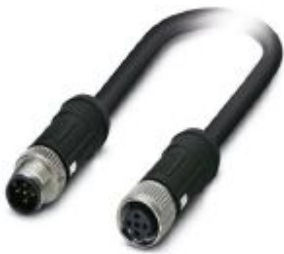
Sensor/actuator cable, 5-position, PE-X halogen-free, black, shielded, Plug straight M12 SPEEDCON, coding: A, on Socket straight M12 SPEEDCON, coding: A, cable length: 5 m, For railway applications
