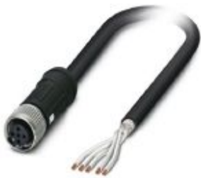
Sensor/actuator cable, 5-position, PE-X halogen-free, black, shielded, free cable end, on Socket straight M12 SPEEDCON, coding: A, cable length: 10 m, For railway applications
