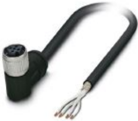
Sensor/actuator cable, 4-position, PE-X halogen-free, black, shielded, free cable end, on Socket angled M12 SPEEDCON, coding: A, cable length: 5 m, For railway applications
