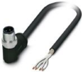
Sensor/actuator cable, 4-position, PE-X halogen-free, black, shielded, Plug angled M12 SPEEDCON, coding: A, on free cable end, cable length: 2 m, For railway applications
