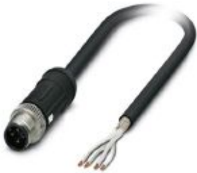
Sensor/actuator cable, 4-position, PE-X halogen-free, black, shielded, Plug straight M12 SPEEDCON, coding: A, on free cable end, cable length: 10 m, For railway applications
