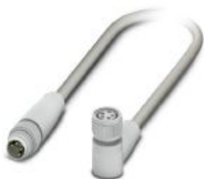
Sensor/actuator cable, 4-position, PP-EPDM halogen-free, gray RAL 7035, Plug straight M8, on Socket angled M8, with 2 LEDs, cable length: 1.5 m, Hygienic design, with plastic knurl
