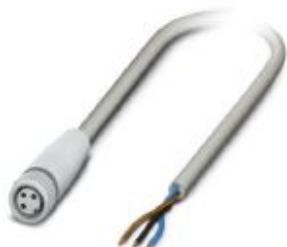
Sensor/actuator cable, 3-position, PP-EPDM halogen-free, gray RAL 7035, free cable end, on Socket straight M8, cable length: 10 m, Hygienic design, with plastic knurl
