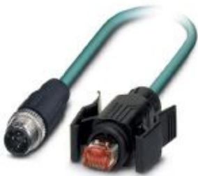
Network cable, Ethernet CAT5 (100 Mbps), 4-position, PUR, water blue RAL 5021, Plug straight M12, on Plug straight RJ45 Clip locking, cable length: 2 m
