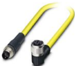
Sensor/actuator cable, 3-position, PVC, yellow, Plug straight M8, on Socket angled M12, coding: A, cable length: 1.5 m
