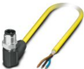
Sensor/actuator cable, 3-position, PVC, yellow, shielded, Plug angled M12, coding: A, on free cable end, cable length: 5 m
