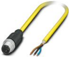
Sensor/actuator cable, 3-position, PVC, yellow, shielded, Plug straight M12, coding: A, on free cable end, cable length: 10 m
