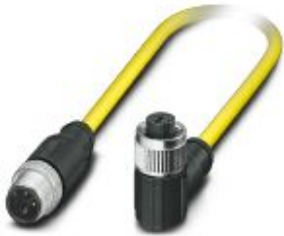
Sensor/actuator cable, 3-position, PVC, yellow, shielded, Plug straight M12, coding: A, on Socket angled M12, coding: A, cable length: 1.5 m
