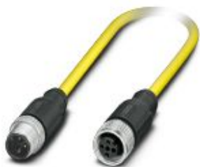
Sensor/actuator cable, 3-position, PVC, yellow, shielded, Plug straight M12, coding: A, on Socket straight M12, coding: A, cable length: 1.5 m
