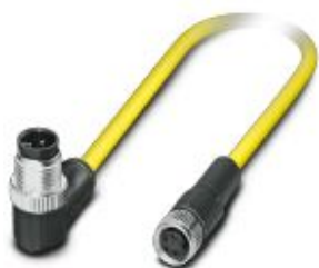
Sensor/actuator cable, 4-position, PVC, yellow, Plug angled M12 SPEEDCON, coding: A, on Socket straight M8, cable length: 1.5 m
