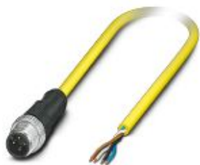
Sensor/actuator cable, 4-position, PVC, yellow, Plug straight M12, coding: A, on free cable end, cable length: 10 m
