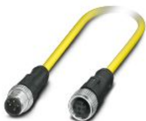
Sensor/actuator cable, 4-position, PVC, yellow, Plug straight M12, coding: A, on Socket straight M12, coding: A, cable length: 0.5 m
