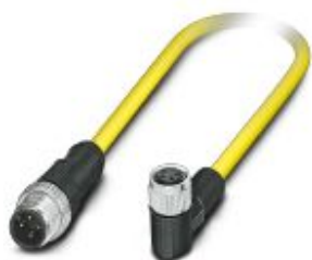
Sensor/actuator cable, 4-position, PVC, yellow, Plug straight M12 SPEEDCON, coding: A, on Socket angled M8, cable length: 0.5 m
