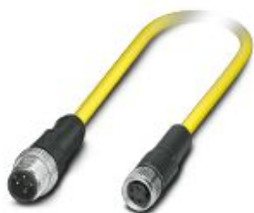
Sensor/actuator cable, 4-position, PVC, yellow, Plug straight M12 SPEEDCON, coding: A, on Socket straight M8, cable length: 1.5 m
