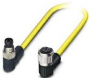
Sensor/actuator cable, 4-position, PVC, yellow, Plug angled M8, on Socket angled M12 SPEEDCON, coding: A, cable length: 0.5 m
