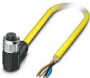
Sensor/actuator cable, 4-position, PVC, yellow, shielded, free cable end, on Socket angled M12, coding: A, cable length: 2 m
