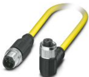
Sensor/actuator cable, 4-position, PVC, yellow, shielded, Plug straight M12, coding: A, on Socket angled M12, coding: A, cable length: 1.5 m
