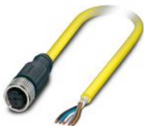
Sensor/actuator cable, 5-position, PVC, yellow, shielded, free cable end, on Socket straight M12, coding: A, cable length: 10 m
