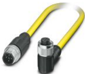
Sensor/actuator cable, 5-position, PVC, yellow, shielded, Plug straight M12, coding: A, on Socket angled M12, coding: A, cable length: 1.5 m
