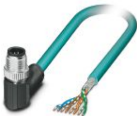
Network cable, Ethernet CAT5 (1 Gbps), 8-position, PUR halogen-free, water blue RAL 5021, shielded, Plug angled M12 / IP67, coding: A, on free cable end, cable length: 2 m
