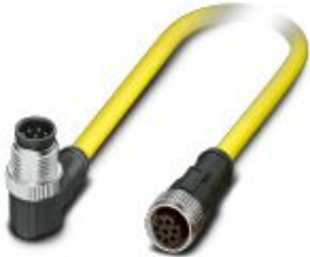
Sensor/actuator cable, 8-position, PVC, yellow, Plug angled M12, coding: A, on Socket straight M12, coding: A, cable length: 0.5 m
