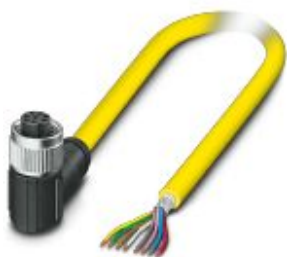
Sensor/actuator cable, 8-position, PVC, yellow, shielded, free cable end, on Socket angled M12, coding: A, cable length: 5 m
