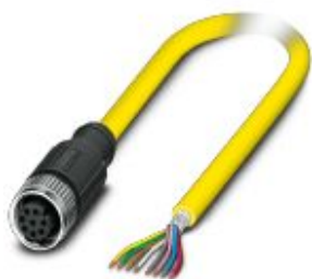
Sensor/actuator cable, 8-position, PVC, yellow, shielded, free cable end, on Socket straight M12, coding: A, cable length: 10 m
