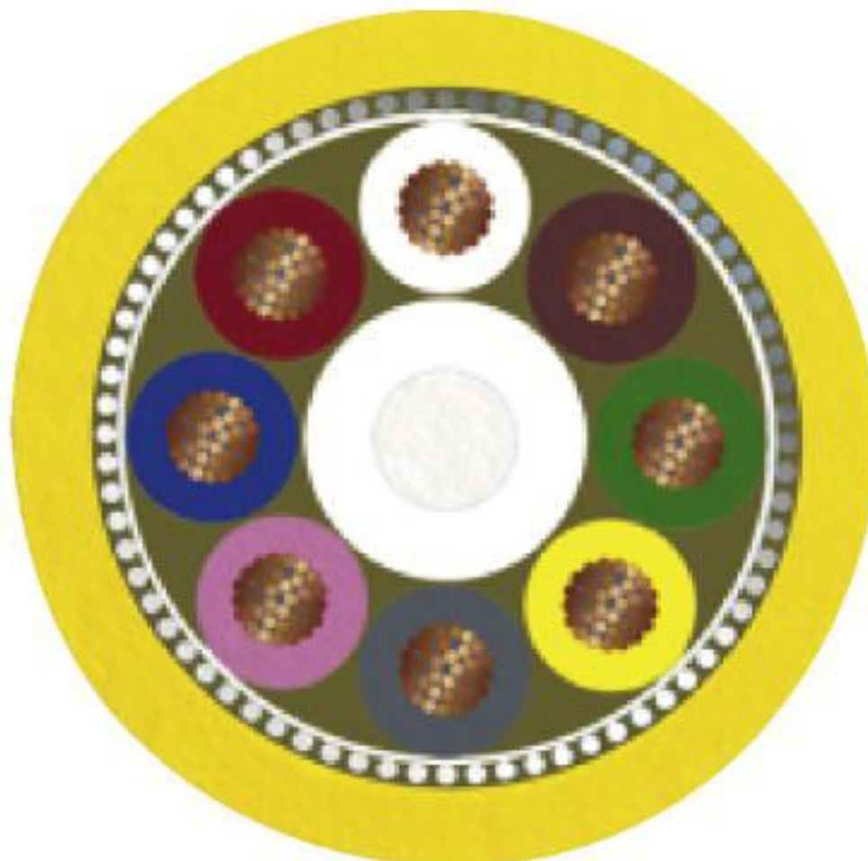
Cable cross section
