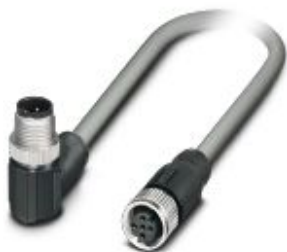
Bus system cable, CANopen®, DeviceNet™, 5-position, PVC, gray, shielded, Plug angled M12 SPEEDCON, coding: A, on Socket straight M12 SPEEDCON, coding: A, cable length: 1.5 m, Connector unshielded
