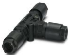
QUICKON T-distributor, gray, 4+PE-pos., 1.0 mm 2 ... 2.5 mm 2 /690 V/20 A, for a cable diameter of 6 mm ... 11 mm with three QUICKON nuts
