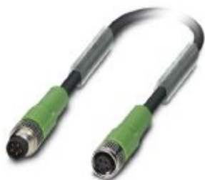
Sensor/actuator cable, 5-position, PUR halogen-free, black-gray RAL 7021, Plug straight M8, coding: B, on Socket straight M8, coding: B, cable length: 0.6 m
