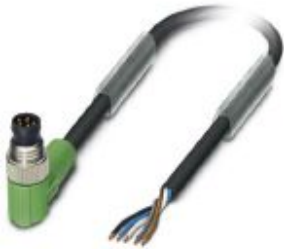
Sensor/actuator cable, 5-position, PUR halogen-free, black-gray RAL 7021, Plug angled M8, coding: B, on free cable end, cable length: 10 m
