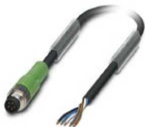
Sensor/actuator cable, 5-position, PUR halogen-free, black-gray RAL 7021, Plug straight M8, coding: B, on free cable end, cable length: 5 m
