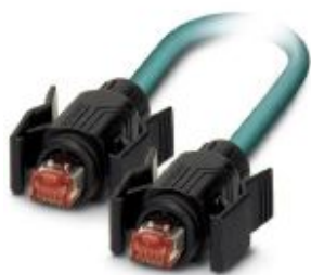
Assembled Ethernet cable, CAT6, shielded, 4-pair, 26 AWG* stranded (7-wire), RAL 5021 (water blue), RJ45 plug/IP67 (black) to RJ45 plug/IP67 (black), line, length: 3 m
