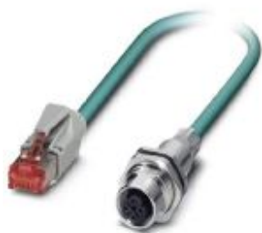
Assembled Ethernet cable, CAT5e, shielded, 2-pair, 26 AWG stranded (7-wire), RAL 5021 (water blue), M12 flush-type socket, rear/screw mounting with SPEEDCON to RJ45 plug/IP20, line, length 1 m
