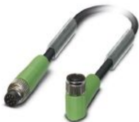
Sensor/actuator cable, 8-position, PUR halogen-free, black-gray RAL 7021, Plug straight M8, on Socket angled M8, cable length: 0.6 m
