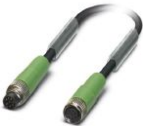
Sensor/actuator cable, 8-position, PUR halogen-free, black-gray RAL 7021, Plug straight M8, on Socket straight M8, cable length: 3 m
