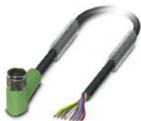
Sensor/actuator cable, 8-position, PUR halogen-free, black-gray RAL 7021, free cable end, on Socket angled M8, cable length: 10 m
